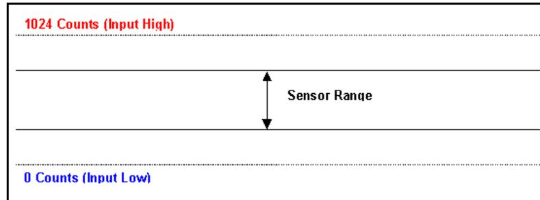
Additionally, the SECM includes software to learn the actual range of the throttle position settings and throttle position sensors in order to take full advantage of the sensor range. Faults are set if the learned values are outside of the normal expected range of the sensor (e.g. APP1AdaptLoMin).
